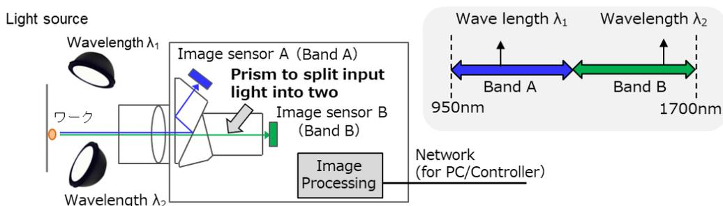
Figure 5 Configuration of spectroscopic prism camera
