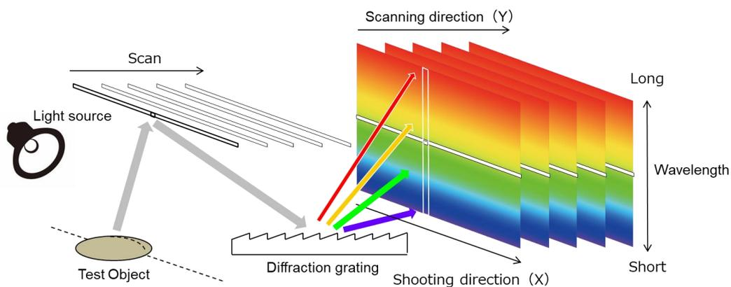
Figure 7 Example of hyperspectral camera configuration
