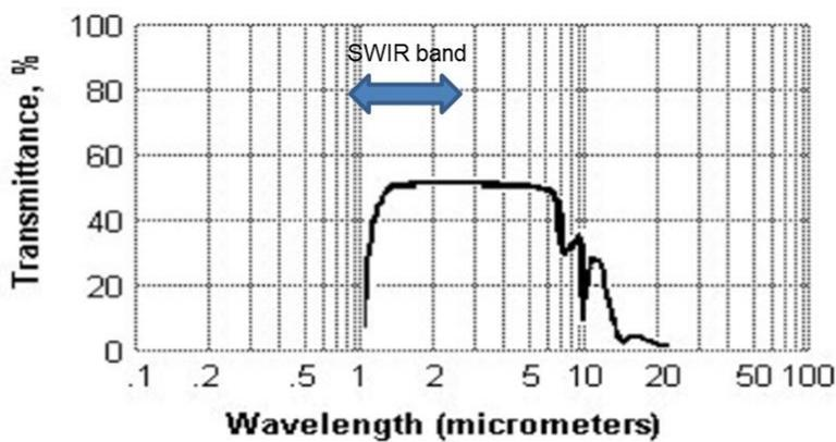
Fig. 2 Transmission of silicon
