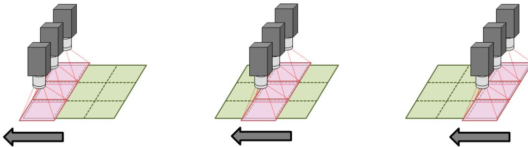
Figure 3a Image shooting process using area cameras
