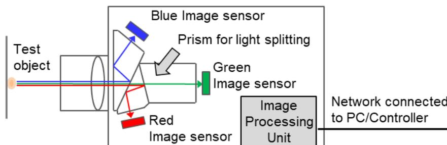
Figure 4 Multicolor line scan camera
