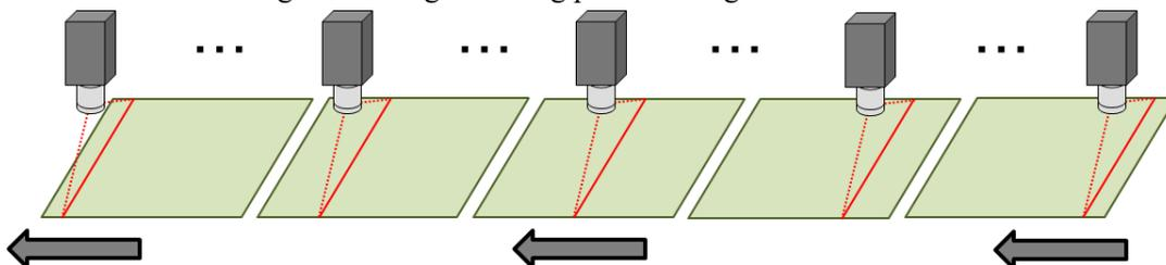
Figure 3b Image shooting process using a line scan camera
