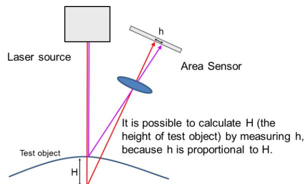
Figure 6b Principle of the inspection using 3D line profile camera
