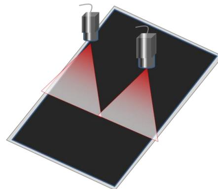
Figure 8b Inspection of LCD panel
